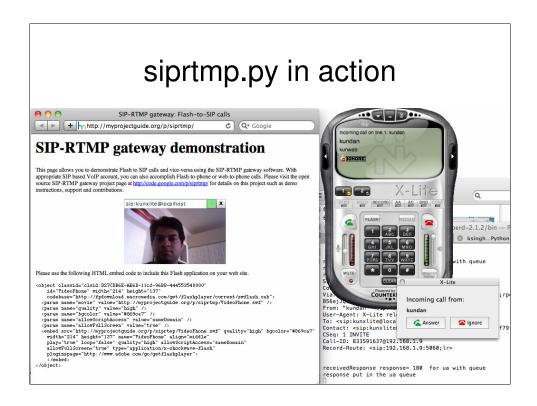
For example, siprtmp is one such project that I have been involved with. The gateway allows a Flash application embedded in a web page to register to SIP server and make or receive SIP calls. The translation mechanism and source code of the gateway is at
