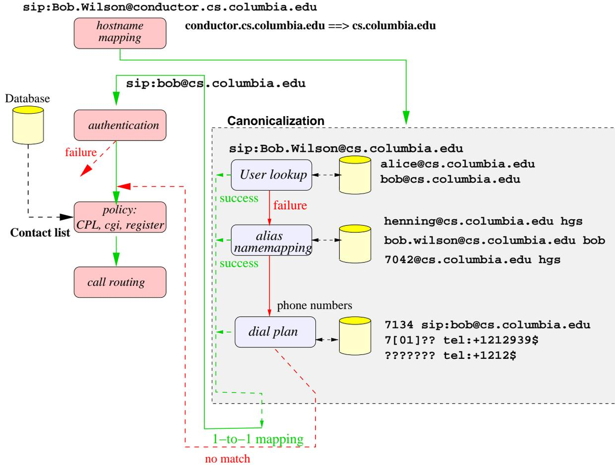
Figure 8: Canonicalization, authentication and routing for a call
