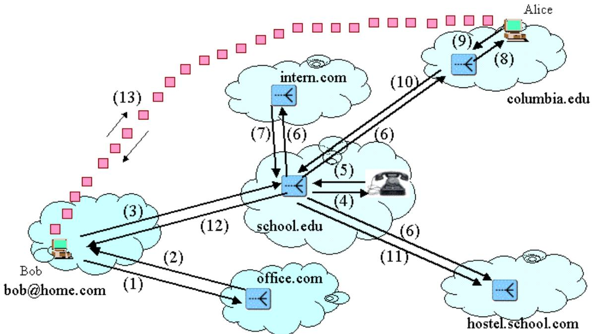
Figure 2: Example SIP call routing
