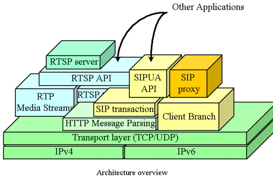
Figure 21: Software Design Modules
