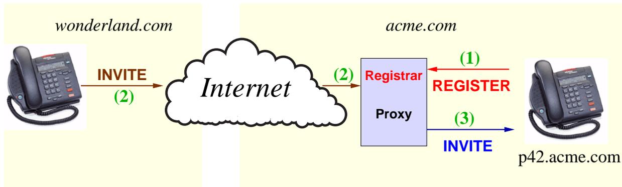
Figure 1: SIP call flow using proxy servers
